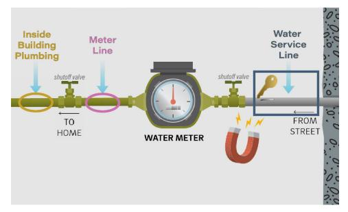
Use your key to scratch the pipe, and try to stick the magnet to the service line.
